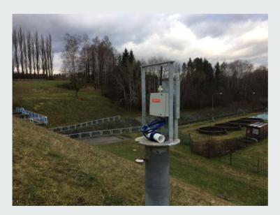
Loadsensing data node installation at the Olešná Dam
