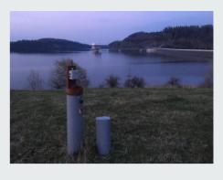
" In spite of being installed in boreholes with steel cover caps or behind the body of the dam with no line of sight to the gateway, the Loadsensing nodes are able to successfully transmit the data without the need for repeaters."
